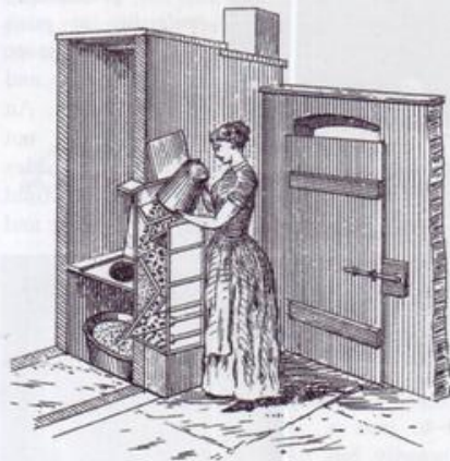
Dry earth closet using ash (Santo Crimp)
