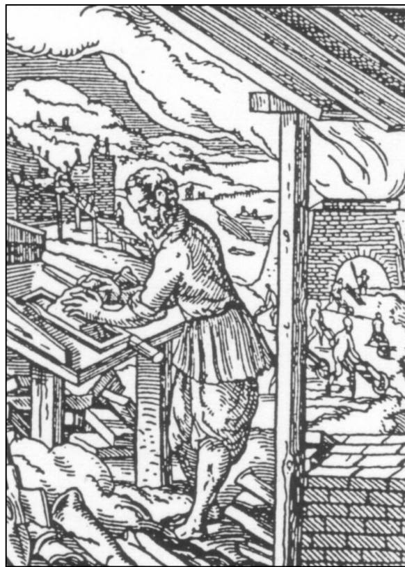
A brickmaker at his bench dashes a clot of clay into his mould.
